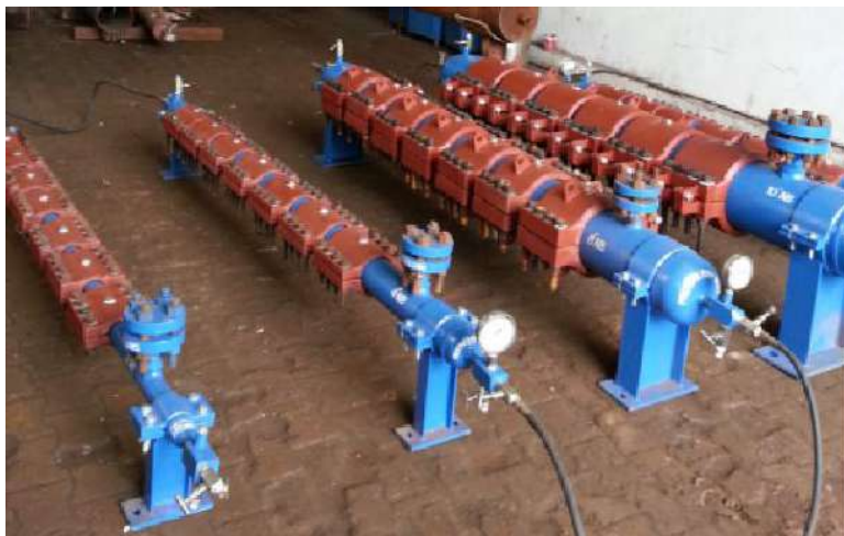
Clamp Hydrostatic testing arrangement
